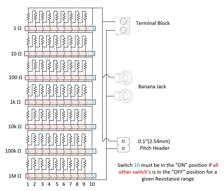
All resistors are 1% tolerance and 0.25 Watt capable.  $1\Omega$  step resolution from  $0\Omega$  to  $10~M\Omega$
